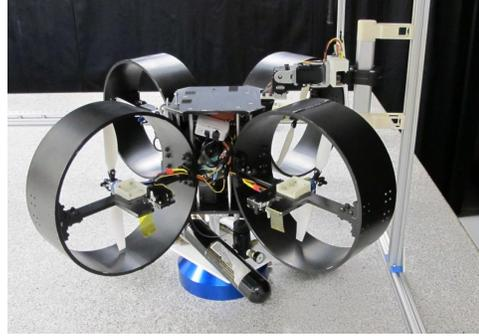
Fig. 1. A prototype of Astrobee grasping an ISS handrail on the top of a micro-gravity simulating surface.
