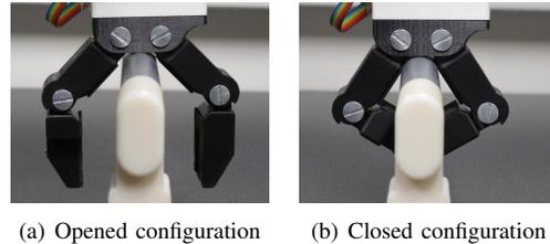
Fig. 2. Snapshot of the Astrobee perching arm grasping an ISS handrail
