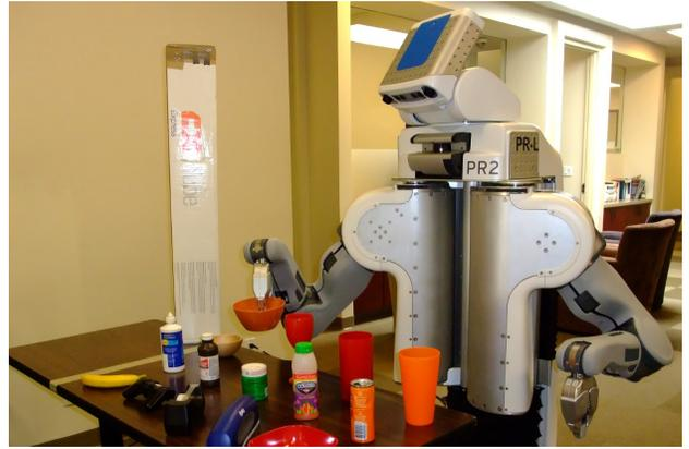
Fig. 2. The PR2 robot performing a grasping task on an object recognized from the model database.
