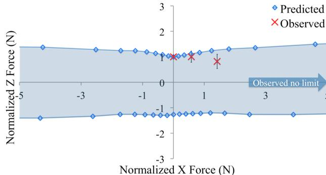
Fig. 5: Normalized forces in the XZ plane that can be resisted by grasp example 1: predicted by our framework, and observed by experiment. In all directions falling between the blue lines (shaded), the prediction framework hit the upper limit of the binary search (arbitrarily set to  $1.0e3$  N). In the direction denoted by “Observed no limit”, the grasp was not disturbed even when hitting the physical limit of the testing setup.
