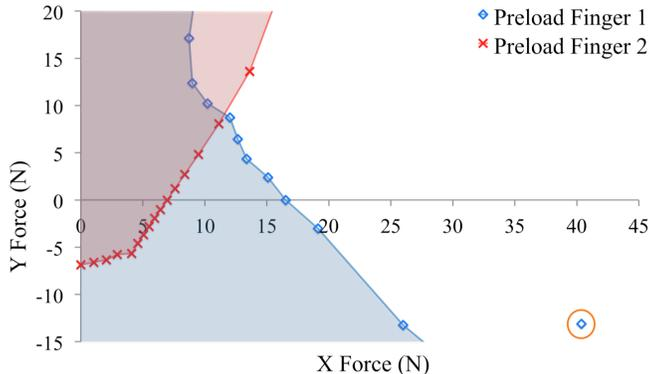
Fig. 7: Forces in an XY halfplane that can be resisted by grasp example 2 (shaded) as predicted by our framework, depending on which finger is preloaded. An outlier prediction is circled in orange.
