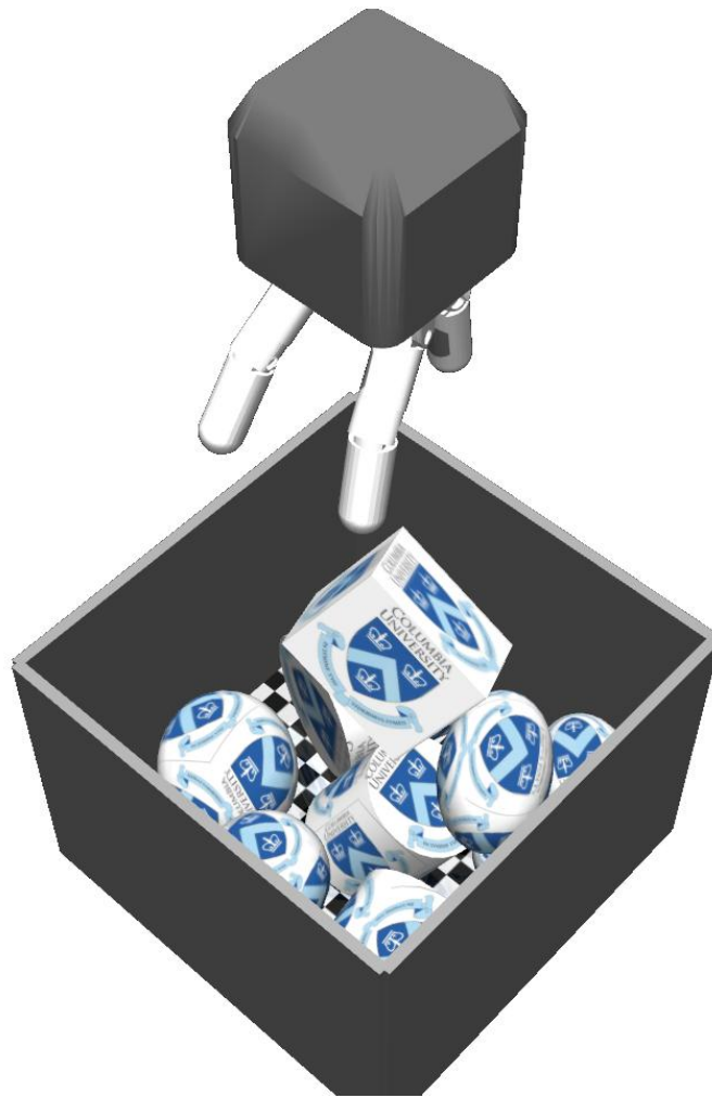
Figure 10.1: The MuJoCo simulation environment for the blind bin-picking task.
