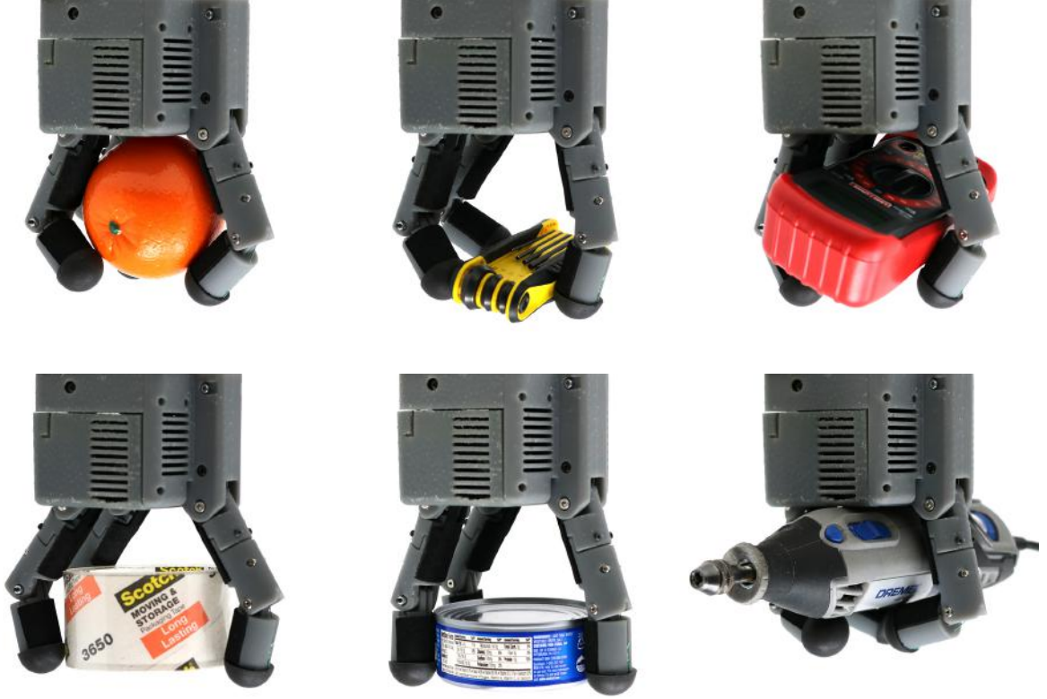
Figure 5.4: The example grasps with different objects.
