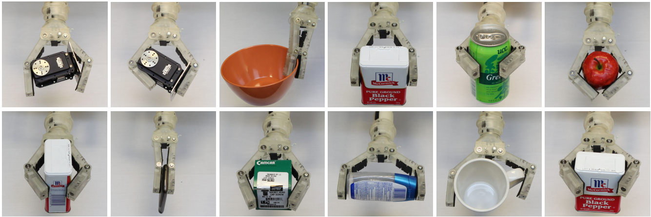
Fig. 12. Examples of grasps executed using prototype gripper.
