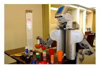
Fig. 2. The PR2 robot performing a grasping task on an object recognized from the model database.
