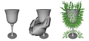
Fig. 1. Grasp planning in simulation on a database model. Left: the object model; Middle: grasp example using the PR2 gripper; Right: the complete set of pre-computed grasps for the PR2 gripper.
