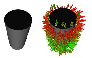
Fig. 3. (Best seen in color) Quantifying grasp robustness to execution errors, from low (red markers) to high (green markers). Note that grasps in the narrow region of the cup are seen as more robust to errors, as the object fits more easily within the gripper.
