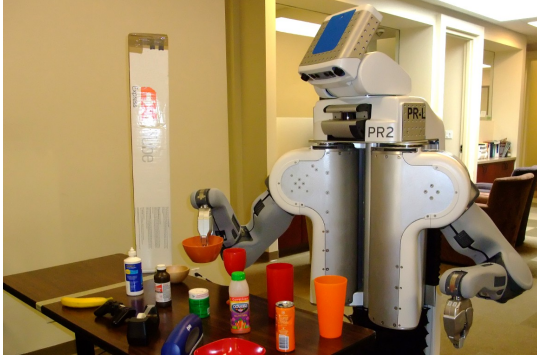
Fig. 7. The PR2 robot performing a grasping task on an object recognized from the model database.
