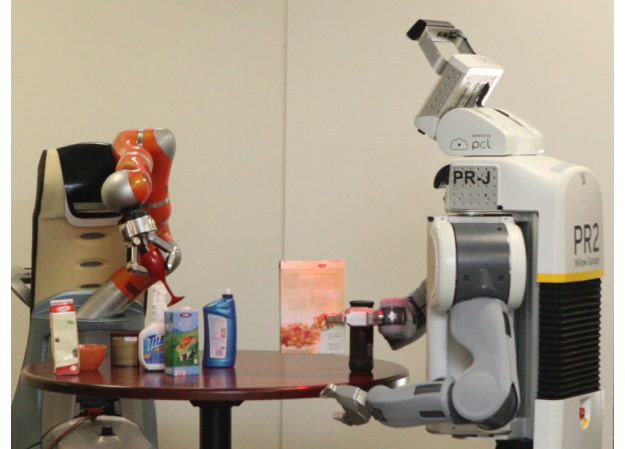
Fig. 1. The PR2 (right) and the Care-O-Bot (left). Both robots are executing a tabletop pick and place task using the approach described in this paper.
