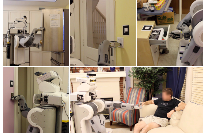
Fig. 1. Examples of robot behaviors constructed using the ROS Commander system and encapsulated as HFSMs: opening a fridge, unlocking with a button, opening a drawer, flipping a light switch, handing off an object.
