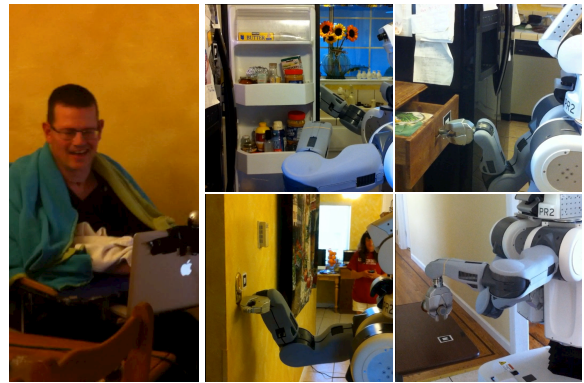
Fig. 5. Behaviors executed by Henry Evans (leftmost image), a person with quadriplegia, at this home: opening a refrigerator, opening a drawer, turning on the lights, and placing an object.
